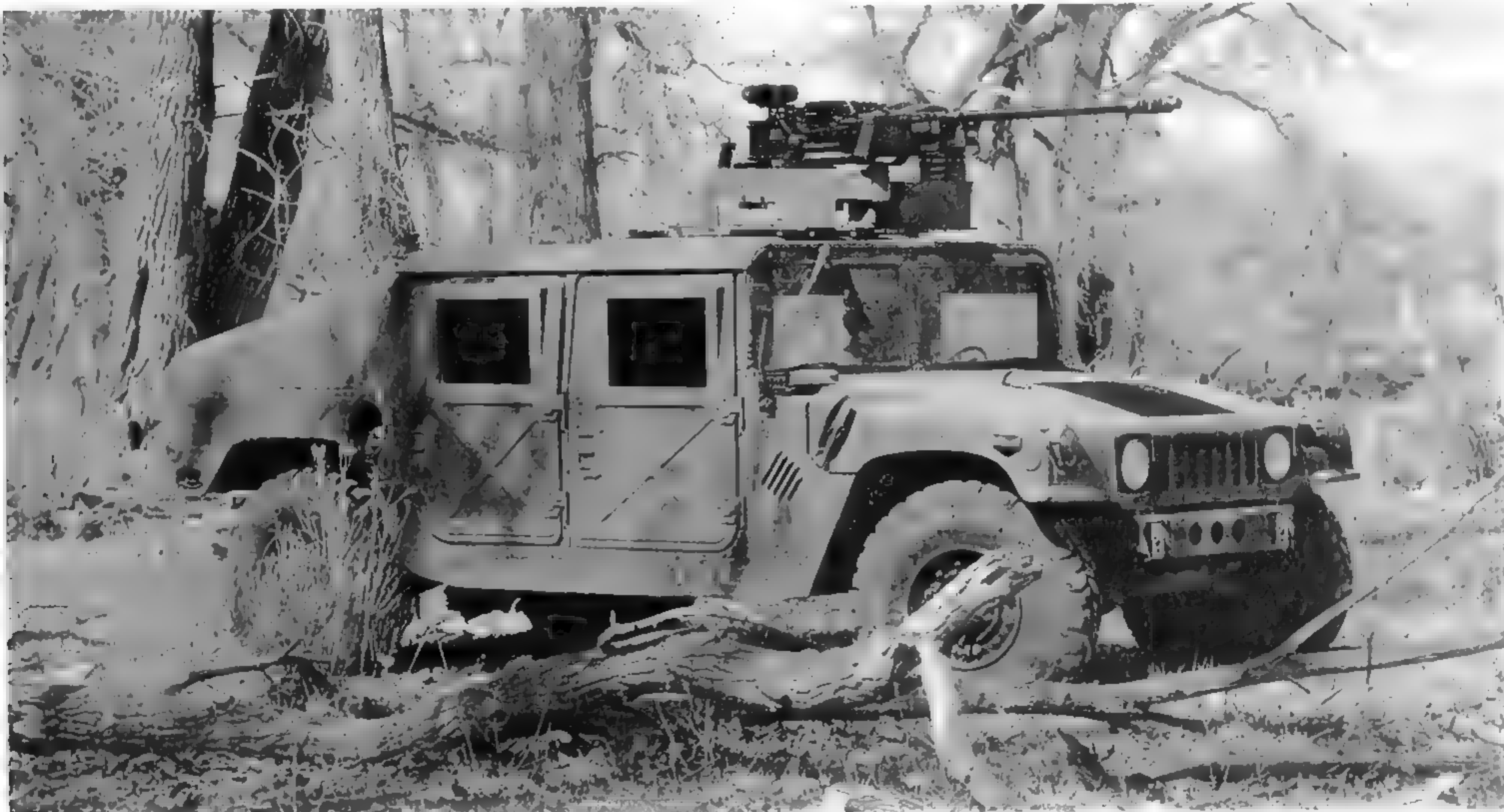
The slant-back M1025 armament carrier is one of the most distinctive members of the HMMWV family. It is protected against splinters, but not opposing direct fire. This vehicle is armed with an MK 19 grenade launcher. (Photo courtesy of AM General Corp.)
